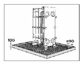
In some cases it may be practical to place the heat exchanger in a drainage box, with capacity for the total volume of the heat exchanger (installation onboard a ship, when processing corrosive liquids, etc.). The outlet of the drainage box should be generously dimensioned, not less than 2" (50mm) diameter.
