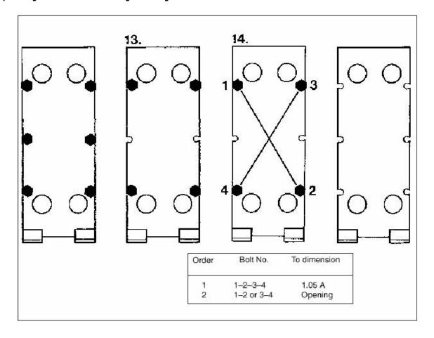
Bolts which are not fitted with bearing boxes are loosened and removed.
