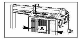
Unless otherwise agreed, WCR delivers the plate heat exchanger ready to be put in service. This means the plate package is tightened to its correct measurement A.
