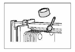
Clean and lubricate the sliding surfaces of the carrying bar.
