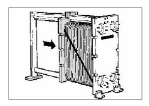
Press the plate assembly together. If the plate pack was marked on the outside double check the plate sequence.
