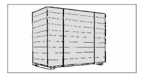
The best solution is often to leave the heat exchanger in the packing case until it is time for installation
