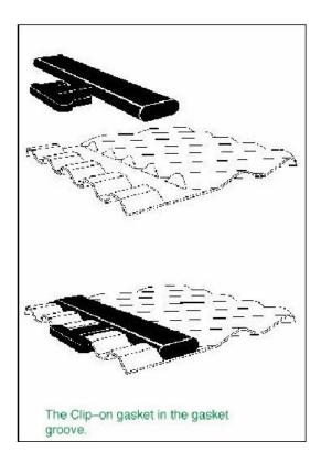
The Clip-on gasket is attached to the plate by two gasket prongs which slip under the edge of the plate to hold the gasket securely in alignment in the gasket groove.
