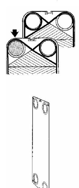
If for instance the thermal program requires that one source of media be lead through more than one group of plates in the plate pack, there will be heat transfer plates with fewer than four holes. In order to prevent the plate from collapsing under the differential pressure, un-punched corners on large plates require extra strong support while the smaller plates are sufficiently strong as stamped.
