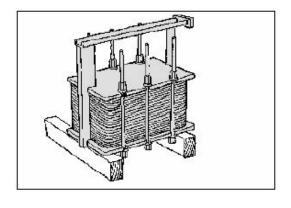
Place the heat exchanger on the timber beams.
