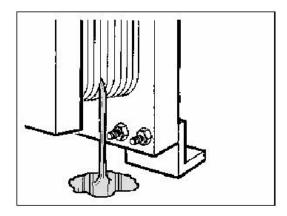
NOTE! On a plate heat exchanger specially designed for high temperature duties, extreme sudden temperature drops may cause a temporary leakage. A typical example is a sudden shutting-off of the hot medium flow. The heat exchanger will normally seal again as soon as the temperatures of the apparatus have stabilized.
