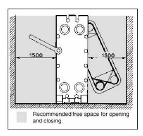
As will appear from the dimension drawing provided by WCR, and from the picture to the left, it is necessary to leave free space around the apparatus to give access and make future service possible. Except for a place to put the plates after removal from the heat exchanger, no further space is required for servicing the PHE.
