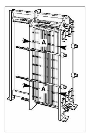
Check the "A" dimension during tightening next to the positions of the tie rods being used. Skewing of the pressure plate during tightening must not exceed 10 mm (2 turns per bolt) across the width and 25 mm (5 turns per bolt) vertically.
