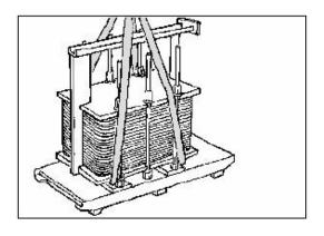
Lift the heat exchanger off the pallet using straps or chains.
