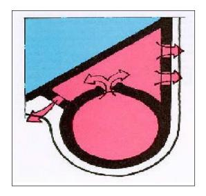
It is important that these openings are not permitted to clog. If clogging of these slots should occur, there exists a risk during a leakage of a local pressure build-up in the clogged region of the plate which could let one medium leak over and mix with the other.
