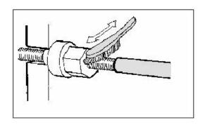
Pull back the plastic covers on the tightening bolts. Brush the threads clean with a steel wire brush.
