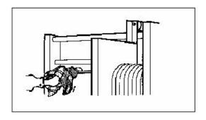
Inspect the sliding surfaces of the carrying bar and wipe clean.
