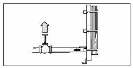
Before starting up for the first time or after a long time of close-down, make sure that the plate pack is compressed to the correct measurement "A"! Check the drawing that is located at the back of this manual.
