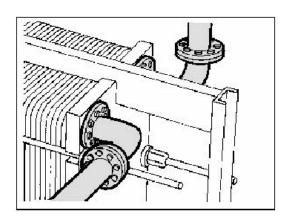
Dismantle any pipe bends connected to the movable plate so that it can be moved freely along the carrying bar.
