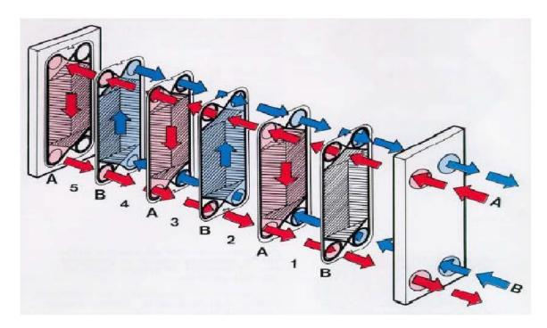
When a package of plates is pressed together, the holes at the corners form continuous tunnels or manifolds leading the media from the inlets into the plate package, where they are distributed into the narrow passages between the plates.
