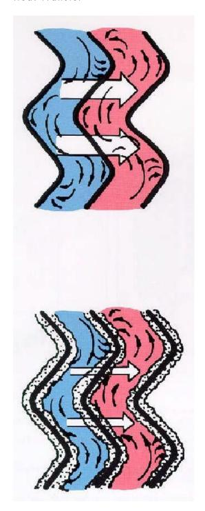
The purpose of the PHE is to transfer heat from one medium to another and the heat passes very easily through the thin wall separating the two media from each other.
