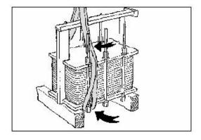
Place straps around one bolt on each side.
