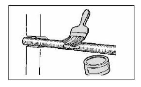
Lubricate the threads with a thin layer of grease.
