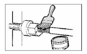
Lubricate the threads with a thin layer of grease.
