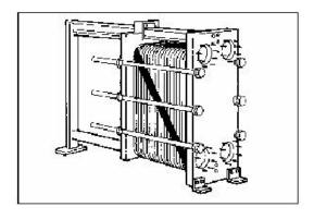
Mark the plate assembly by drawing a diagonal line as shown, or number the plates in order.
