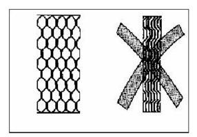
Make sure the plates are correctly assembled. The edges should form a "honeycomb" pattern.
