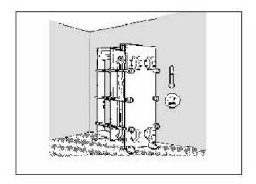
Preferably, the heat exchanger should be stored inside at room temperatures of 60- 70F (15-20C) and humidity around 70%
