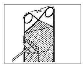
Hydrocarbon-based deposits may be removed by using a soft brush and a Paraffinc or Naphta-based solvent (e.g. Kerosene).
