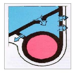
As already demonstrated, the two media are kept separated by the ring and field gaskets. To prevent intermixing of the media in the corner areas where field and ring gaskets are very close to each other, the linking pieces have a number of slots, opening the area between the field and ring gaskets to the atmosphere. Any leakage of media across either gasket therefore escapes from the heat exchanger through the slots.
