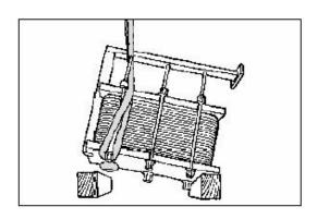
Lift the heat exchanger from the timber beams.
