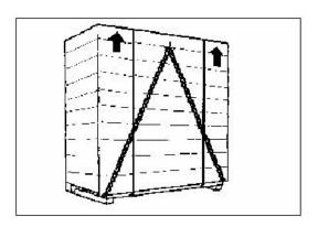
When lifting the unopened packing case (or skid) please observe the markings on the case indicating where to place lifting hooks. The center of gravity is important and is marked on the topside of the case. The actual center of gravity is located on the vertical line directly below this mark. WCR generally advises customers in advance on how the heat exchanger has been placed inside the crate.
