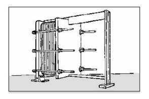
Lower the heat exchanger to horizontal and place on floor.
