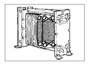
Check that all the sealing surfaces (i.e. surfaces in contact with the heat transfer medium) are clean.
